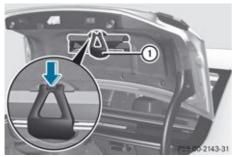
Press warning triangle holder Oup in the direction of the arrow, open it and remove the warning triangle.
