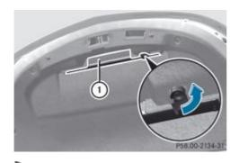
Turn the catch 90° in the direction of the arrow and remove warning triangle ①.
